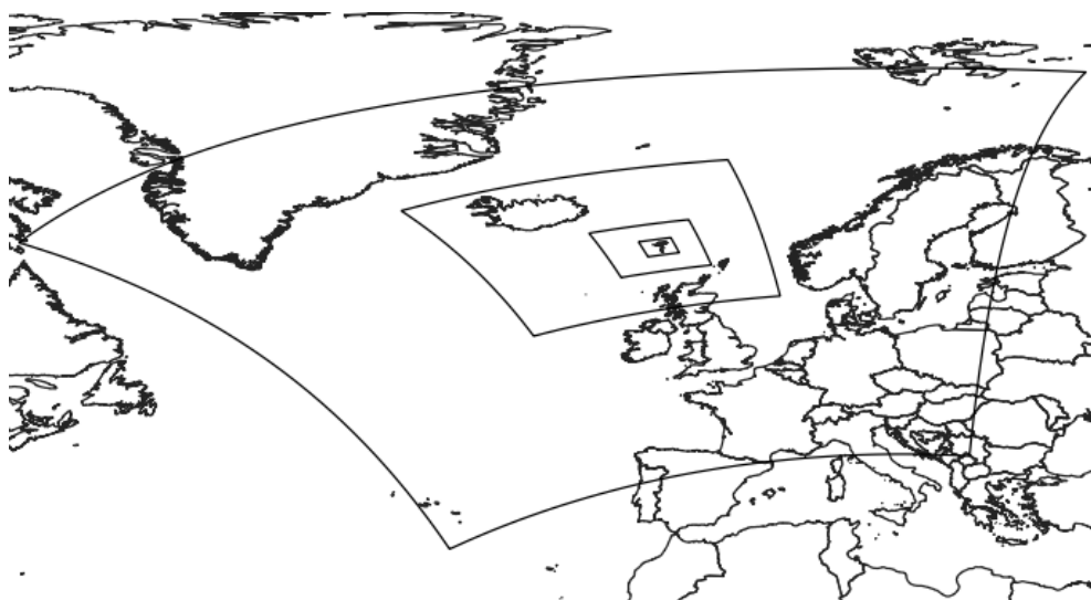
Figure 13 The 4 domains used for the 1km simulation. The horizontal resolution is 27km, 9km, 3km and 1 km respectively
